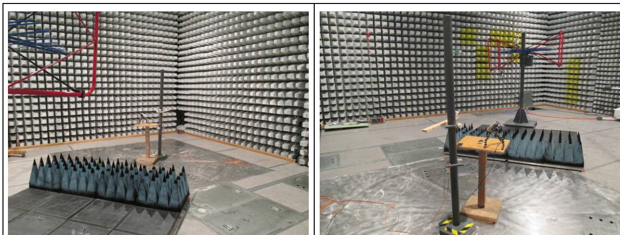
Figure 6-15: test setup for radio frequency electromagnetic fields 80 MHz to 1000 MHz
